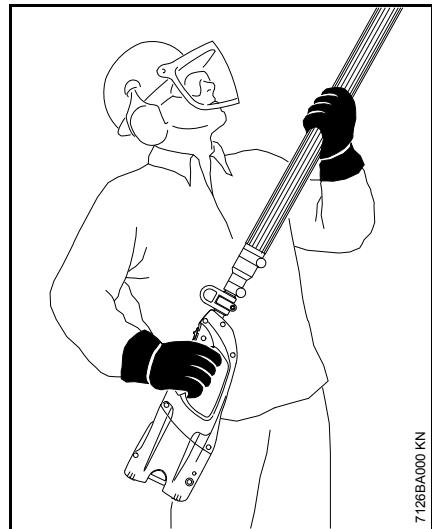
Wrap your fingers and thumbs around the handles. Left hand on handle hose on shaft, right hand on control handle.
